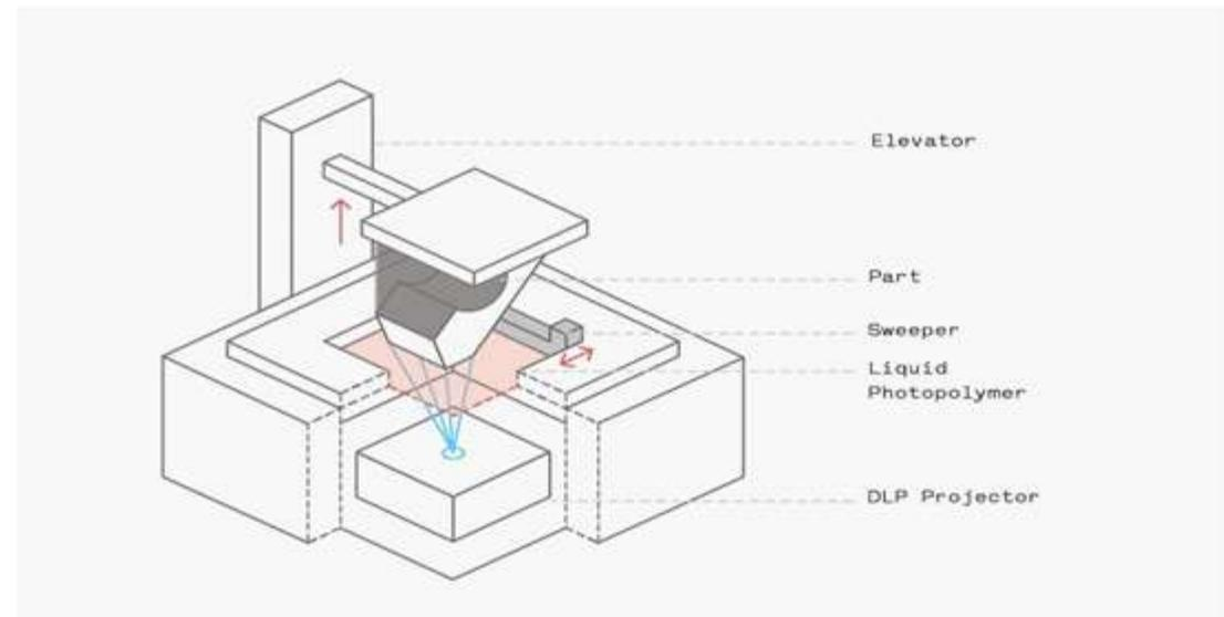
Schematic of a DLP printer
