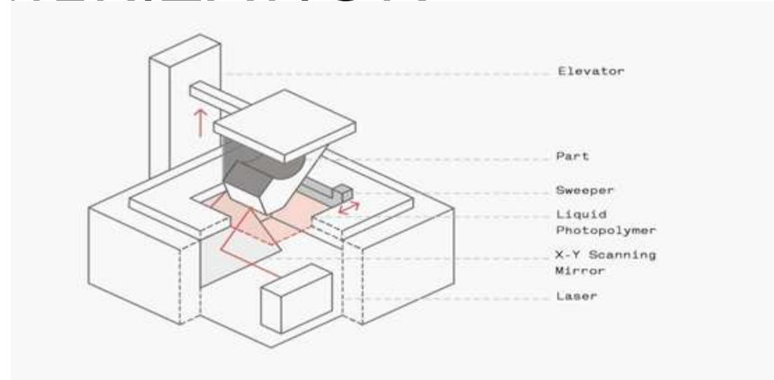
Schematic of a SLA printer
